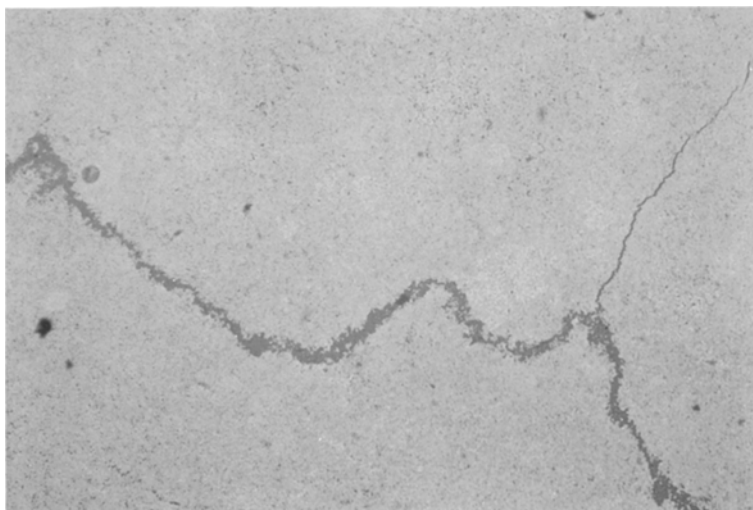
Figure 1 Polished section of a synthetic hollandite showing cracks ranging in width from 2 to 100 \mu\text{m} completely penetrated by plastic. ( \times 56.25 ).
